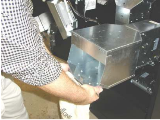
MC920 Bulk Dumping a 10K Hopper
